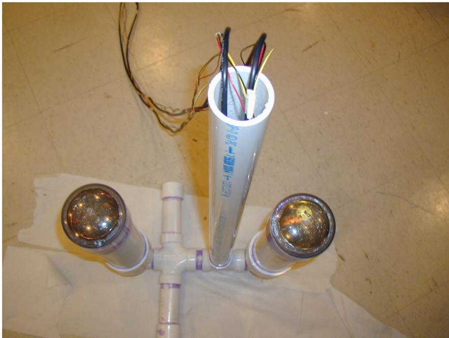
**Figure 5.4** PVC PMT Housing.
